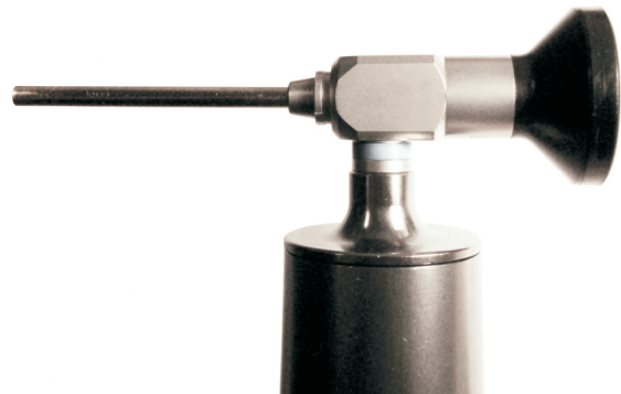
LED LIGHT SOURCE COUPLED WITH RIGID BORESCOPE
